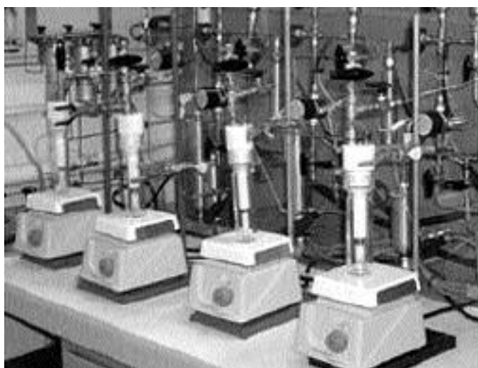
The center conducts useful research for industrial clients. Among its instruments are these computer-controlled low-pressure reactor systems.
